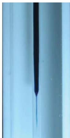
Figure 2. Miscible displacement pattern in the non-reactive case at t = 480 s under the conditions of At = 0.998 , Pe = 3300 , and F = -200 .
